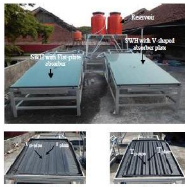
Figure 5 Solar water heating system with (a) flat-plate absorber plate (b) V-shaped absorber plate.
